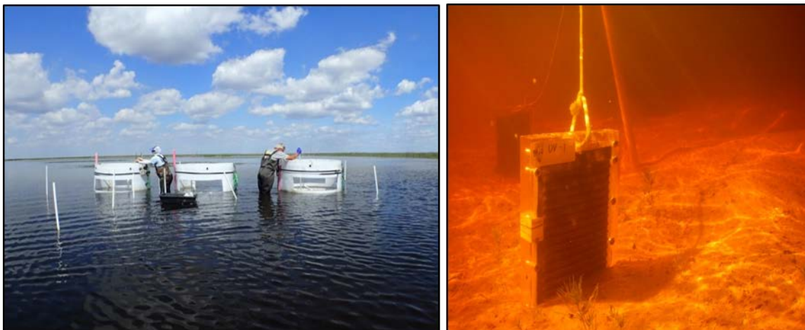
Figure 14. Flux chambers installed in the outflow region of STA-2 FW 3, during a chamber closure/monitoring event (left) and an installed porewater equilibrator (right).
