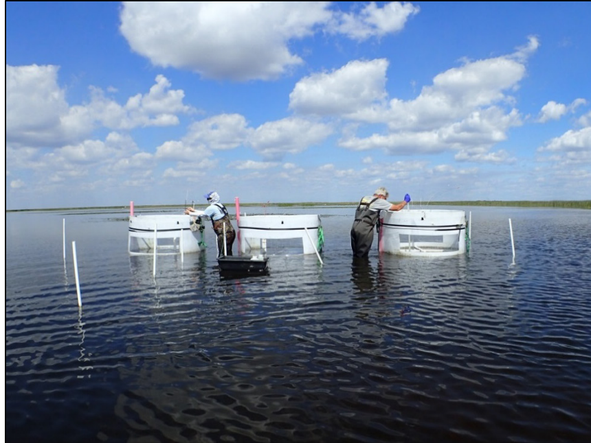
Figure 11. Flux chambers installed in the outflow region of STA-2 FW 3, during a chamber closure/monitoring event.
