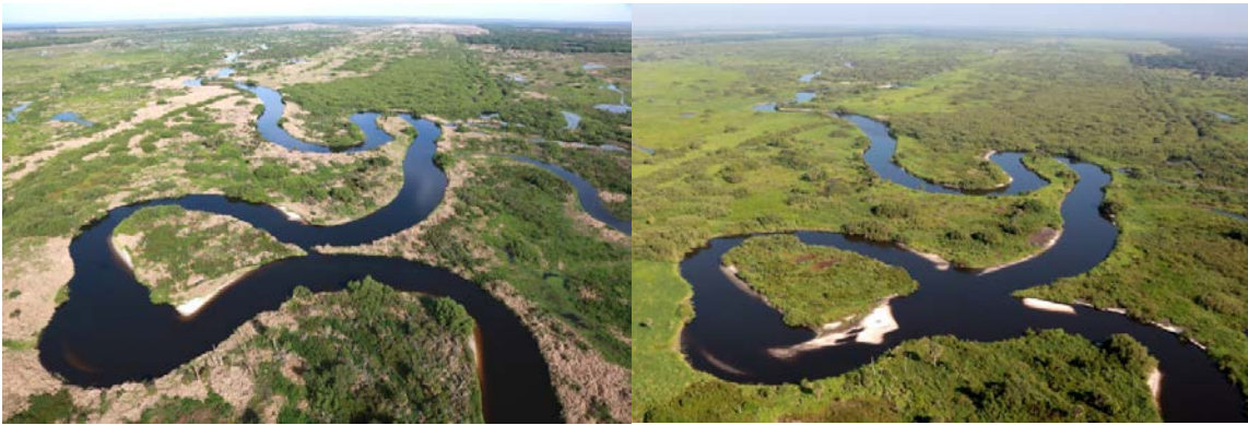
Figure 9-31. A newly formed meander cutoff (left) created an island in the former Micco Run in the Kissimmee River Phase I restoration area. The cutoff began to form in mid-March 2014, has continued widen through May 2015 (right), and is now the main conduit of flow.
