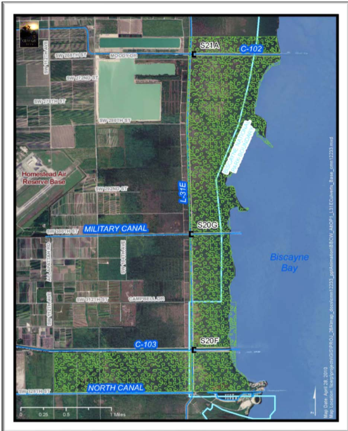
Figure B-2. BBCW L-31E culverts project area (green pattern) and monitoring structures.
