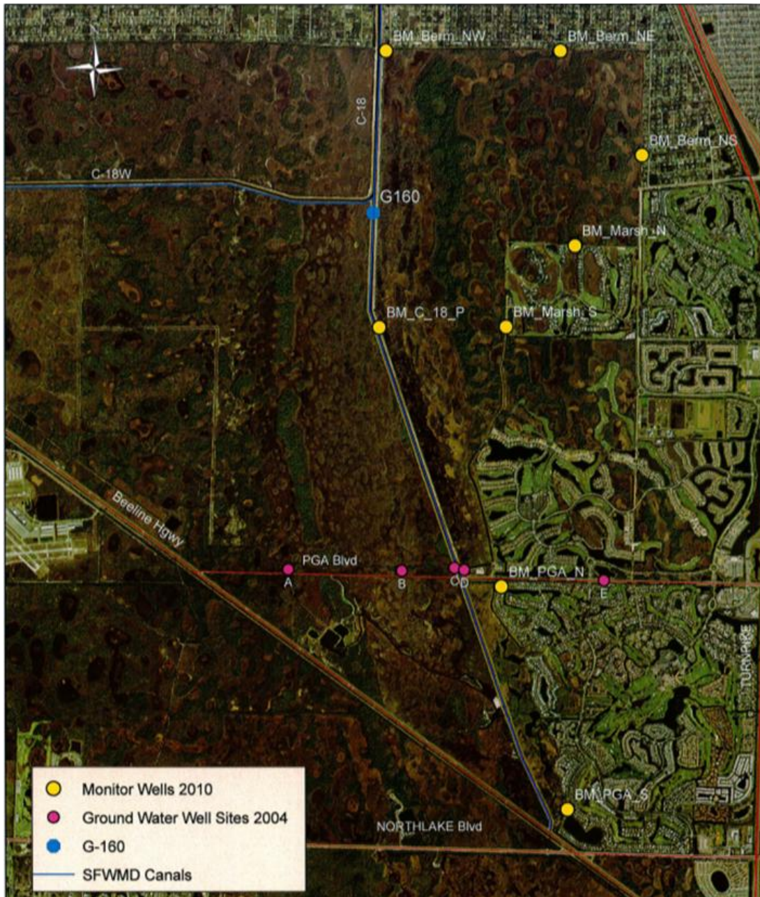
Figure 2. Groundwater monitoring wells in the vicinity of G-160/161.
