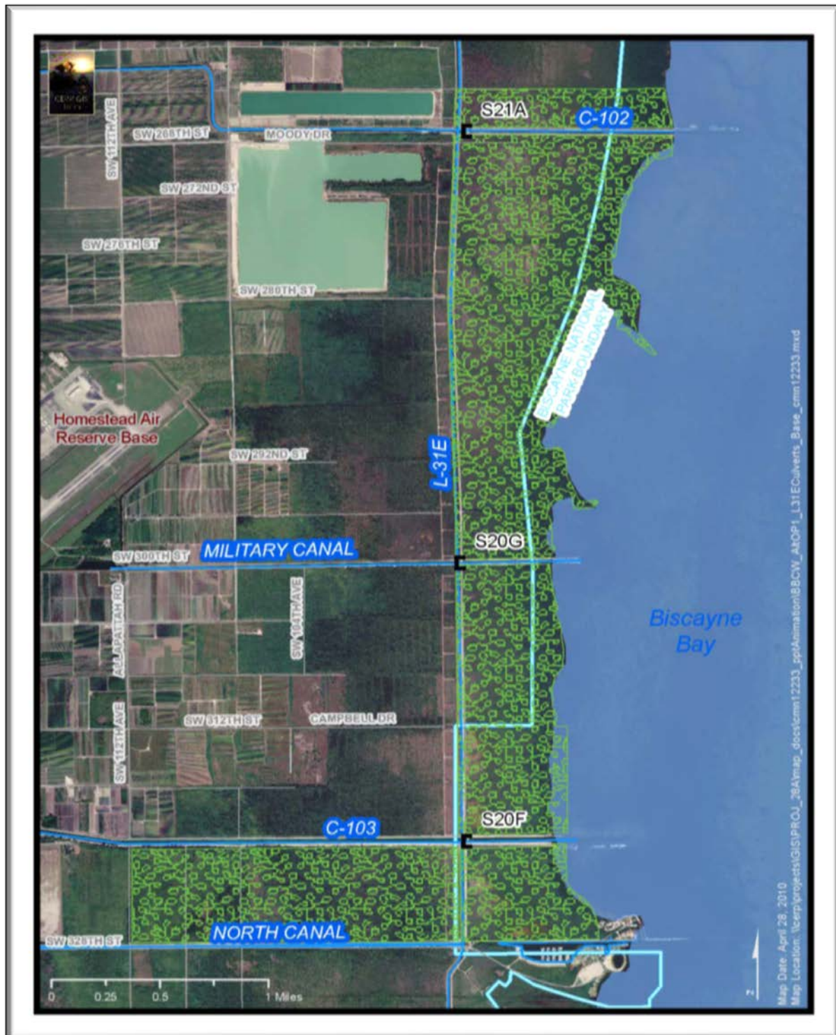
Figure 3- Biscayne Bay Coastal Wetlands, L -31E Culverts Project area (green pattern) and monitoring structures.
