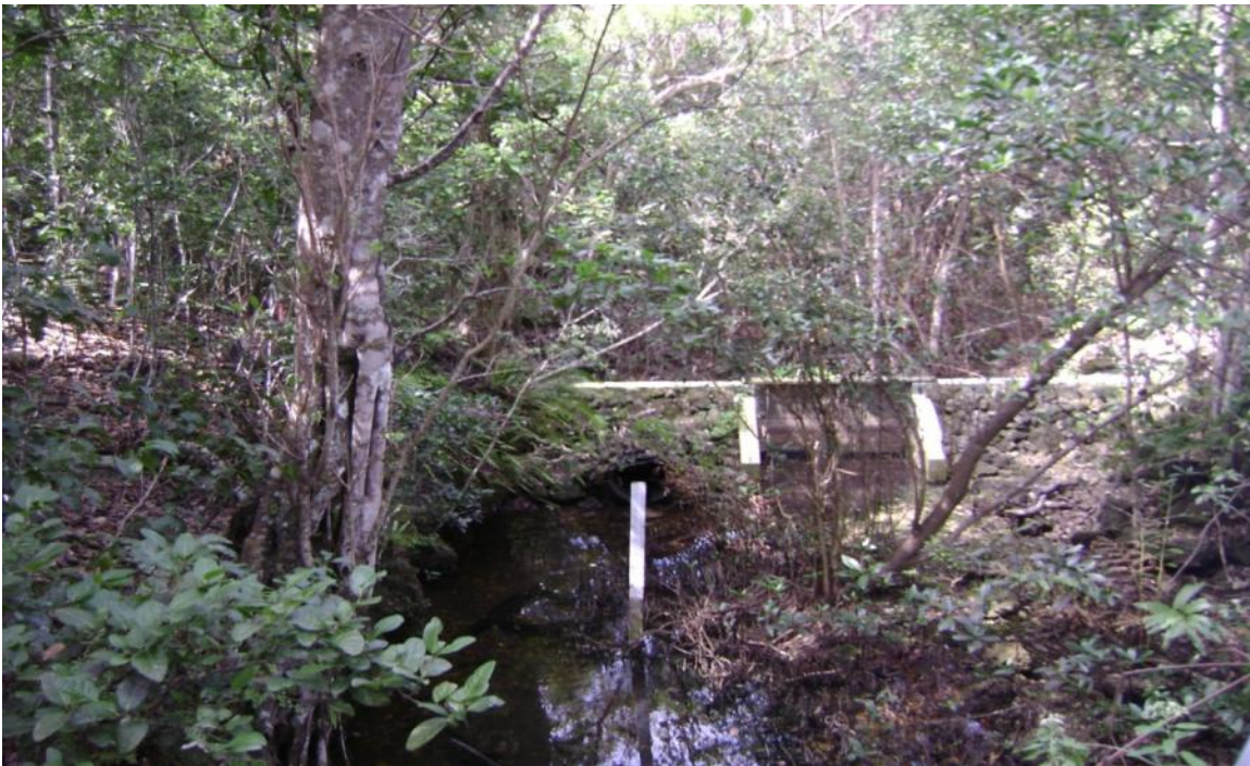
Figure 12- Photo of Existing Wetland Stage (Staff Gauge) Station 3 Monitoring Station within Cutler Creek downstream of the weir
