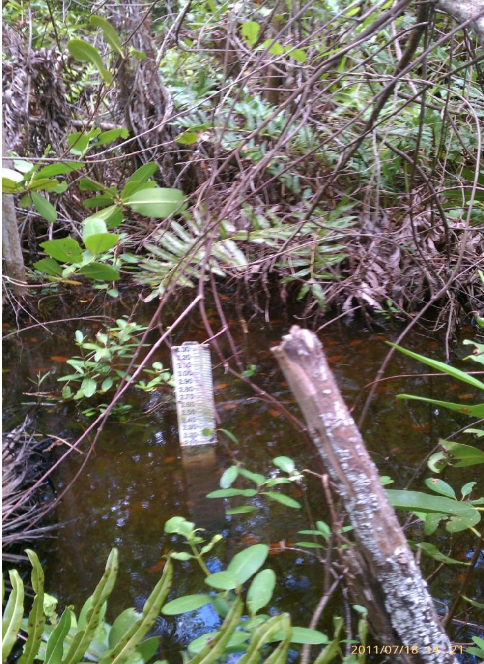
Figure 14- Photo of Existing Wetland Stage (Staff Gauge) Station1 Monitoring Station within Cutler Creek upstream of the weir
