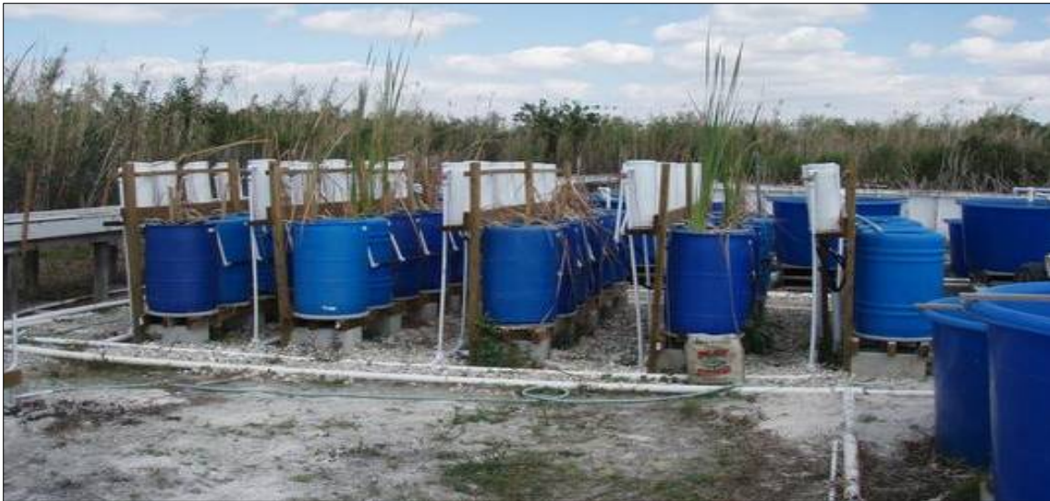
Figure 6-30. Set-up of the flow-through Supplemental Sediment Core Study conducted at the South Advanced Technology Treatment Site of STA-1W (photo by DB Environmental, Inc., under contract to the SFWMD).
