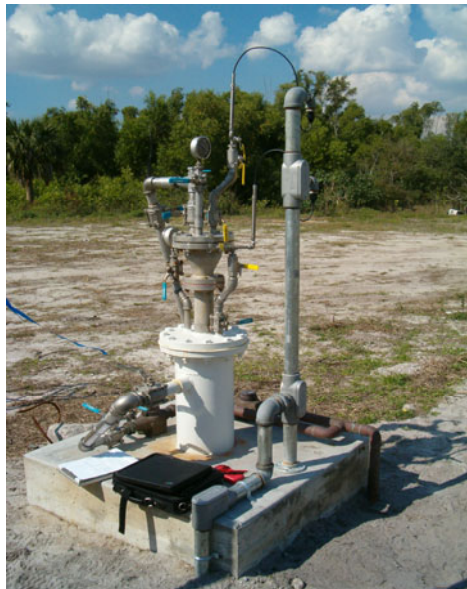
Figure 59. The In-Situ Level Troll 500 transducer connected to a Floridan Aquifer well.
