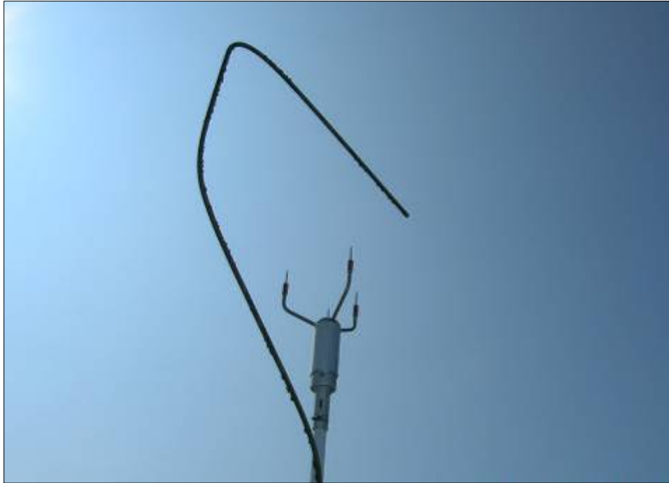
Figure 8. A Vaisala WS425 ultrasonic wind sensor at weather station L006.
