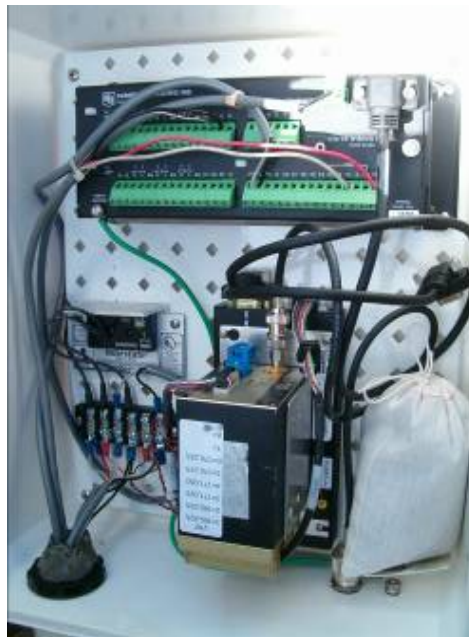
Figure 57. A Campbell Scientific® CR10 data logger (attached to pressure transducer in a non-artesian well).
