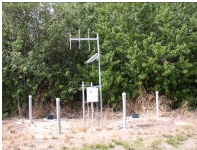
Figure 60. A non-artesian well site connected via telemetry.
