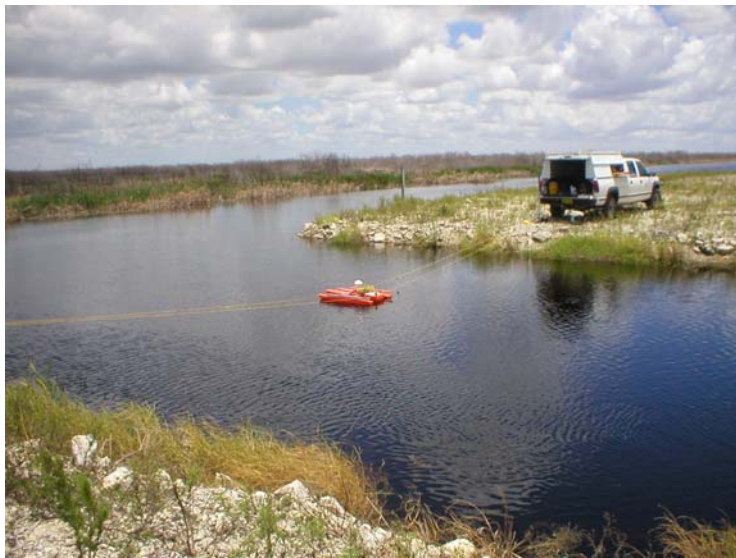
Figure 48. Flow measurement with a StreamPro.
