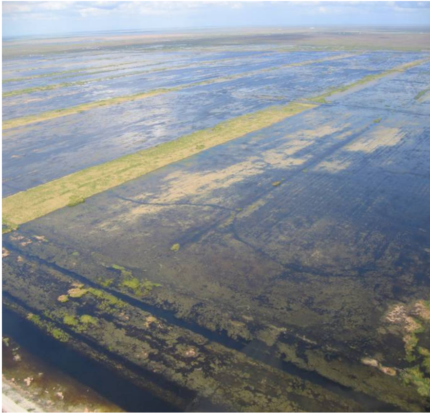
Figure 5-36. Vegetation strips, consisting of emergent plants, serve as wind and wave barriers to fortify the SAV communities against large storm events.
