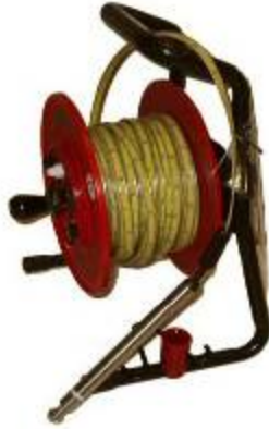
Figure 61. Electronic well sounder used for measuring groundwater levels.
