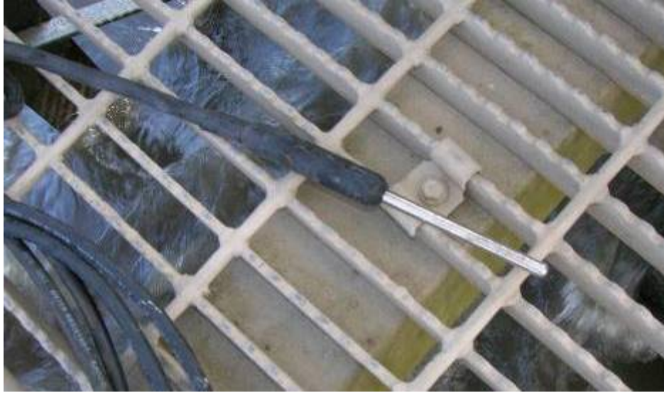
Figure 14. A Campbell Scientific Thermistor temperature probe at weather station L006.
