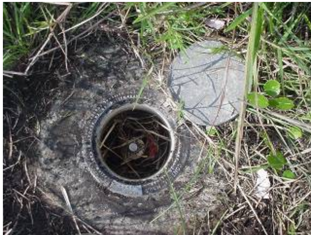
Figure 62. An un-instrumented groundwater monitoring well (typically measured with a well sounder).
