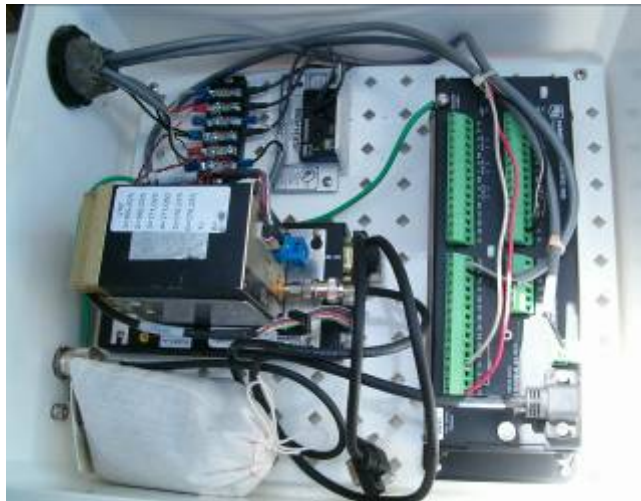
Figure 57. A Campbell Scientific® CR10 data logger (attached to pressure transducer in a non-artesian well).
