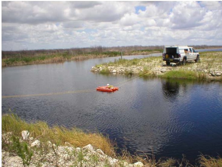
Figure 48. Flow measurement with a StreamPro.
