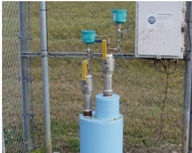
Figure 59. Rittmeyer® pressure transducers connected to a Floridan Aquifer System dual-zone well.
