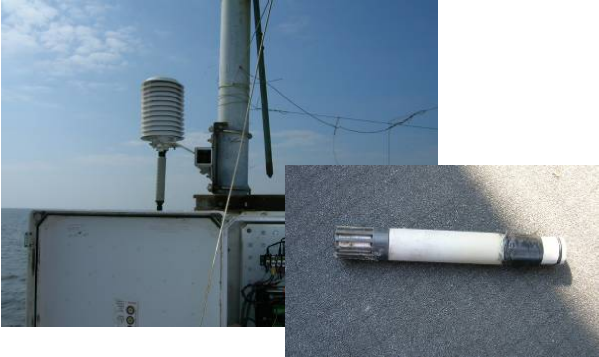
Figure 9. An air temperature and relative humidity probe at weather station L006.
