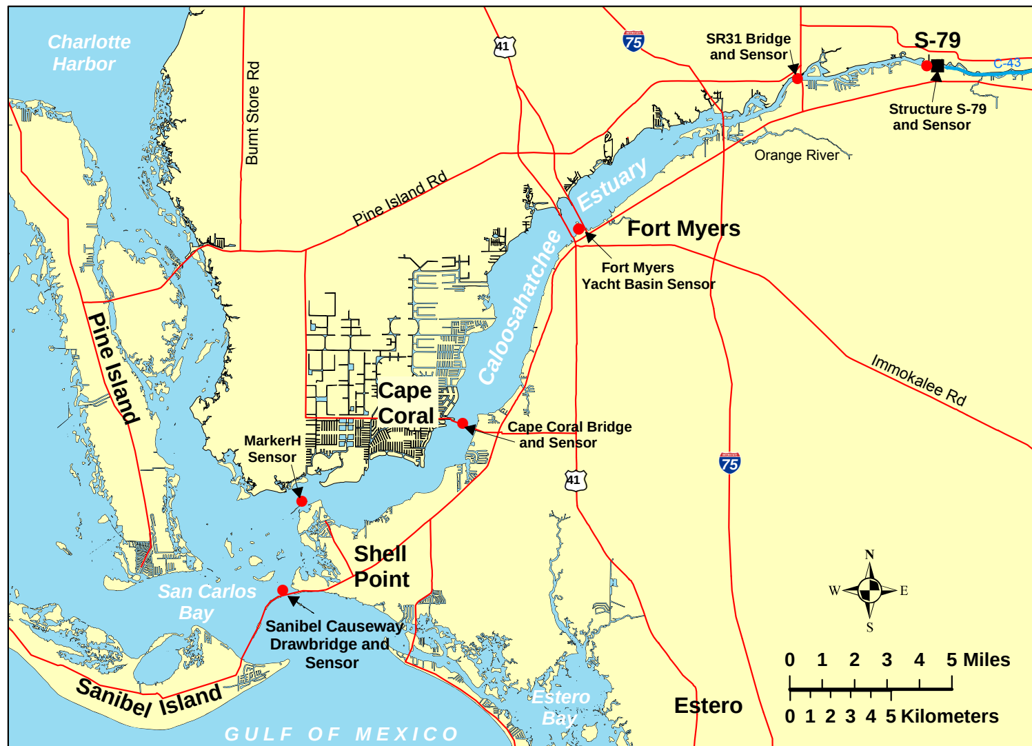
Figure 12-40. Caloosahatchee Estuary salinity sensors and important landmarks.
